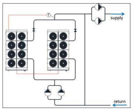
With Master/Slave control is possible to balance the working hours of the compressors enhancing reliability and extending the life of the system
