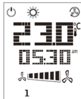
Ventilation mode, heating
